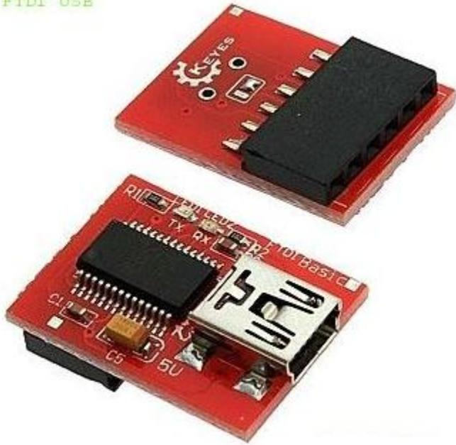
This module provides users with alternatives of module power supply. Three solder joints in the diagram below, the bottom one is for 5V, upper one for 3.3 V. Users can choose power supply according to corresponding USB's power supply voltage. Just weld it on with soldering iron. USB to serial port can be used together with Arduino mini. Plug Arduino mini to corresponding pins of the convert module, you can then upload arduino program to Arduino mini.
